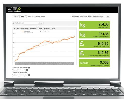
to help you appreciate your end-of-life food generation patterns and manage the efficient use of your Waste<sub>2</sub>O. The food waste reporter uses sensors placed within the Waste<sub>2</sub>O to monitor and record the end of fife food waste levels within the digester over time. This tool can be found at <u>www.waste2-0.com</u>
