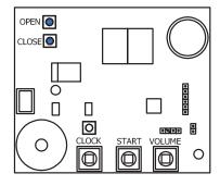
5.2.21 To adjust the clock: Press the CLOCK (left) button. The display will show the hour (24hr clock). Hold for 5 seconds and until the current hour is displayed. You will hear a ticking sound as the display advances.
