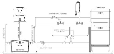
INSTALLATION EXAMPLE - LOW FOG PRODUCING OPERATION - ONE BIOCEPTOR INSTALLED
