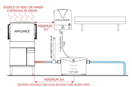
Be sure that the delivery tube trap is properly supported and not stretched. The tube should be a smooth run and clipped in place.
