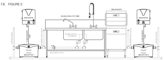
INSTALLATION EXAMPLE - HIGH FOG PRODUCING OPERATION - TWO BIOCEPTORS INSTALLED
